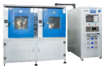
大水泵耐久测试台 Main Water Pump Durability Test Bench
